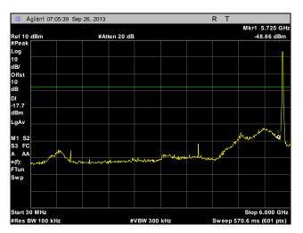
Plot 250. Conducted Spurious Emissions, High Channel, 20 MHz, Port 2, 30 MHz - 6 GHz
