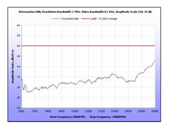
Plot 202. Radiated Spurious Emissions, High Channel, 40 MHz, 6 GHz - 18 GHz, Average, 21 dBi
