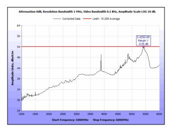
Plot 140. Radiated Spurious Emissions, High Channel, 20 MHz, 1 GHz - 6 GHz, Average, 21 dBi
