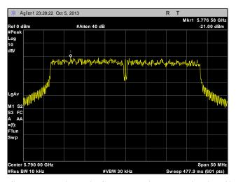
Plot 330. Peak Power Spectral Density, Mid Channel, Point to Multi-Point, 40 MHz, Port 2, 28 dBi
