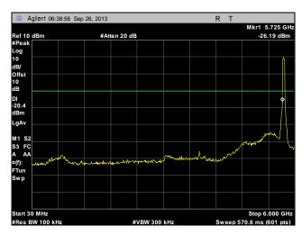
Plot 252. Conducted Spurious Emissions, Low Channel, 40 MHz, Port 1, 30 MHz - 6 GHz
