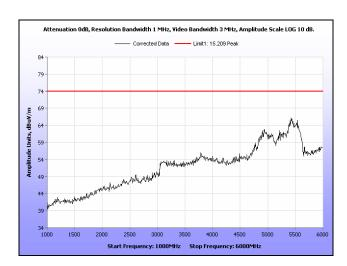
Plot 213. Radiated Spurious Emissions, High Channel, 40 MHz, 1 GHz - 6 GHz, Peak, 23 dBi
