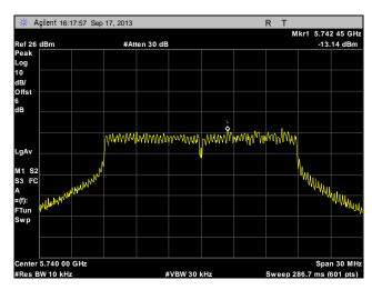
Plot 290. Peak Power Spectral Density, Low Channel, Point to Multi-Point, 20 MHz, Port 2, 19 dBi
