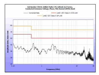
Plot 13. Conducted Emissions, 15.207(a), Neutral Line, Mid Channel, 20 MHz
