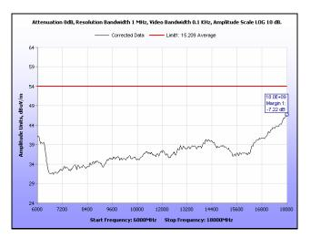
Plot 118. Radiated Spurious Emissions, High Channel, 20 MHz, 6 GHz - 18 GHz, Average, 16 dBi
