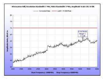
Plot 217. Radiated Spurious Emissions, Low Channel, 40 MHz, 1 GHz - 6 GHz, Peak, 28 dBi
