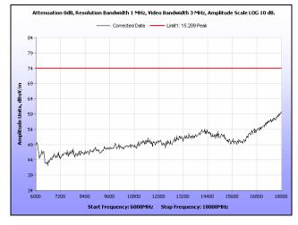
Plot 203. Radiated Spurious Emissions, High Channel, 40 MHz, 6 GHz – 18 GHz, Peak, 21 dBi
