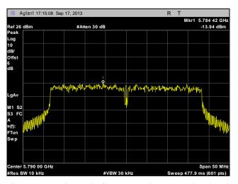
Plot 306. Peak Power Spectral Density, Mid Channel, Point to Multi-Point, 40 MHz, Port 1, 19 dBi
