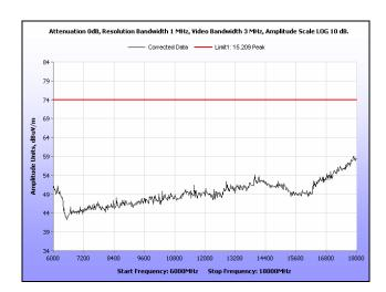
Plot 111. Radiated Spurious Emissions, Low Channel, 20 MHz, 6 GHz - 18 GHz, Peak, 16 dBi
