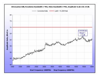
Plot 161. Radiated Spurious Emissions, Mid Channel, 20 MHz, 1 GHz - 6 GHz, Peak, 28 dBi
