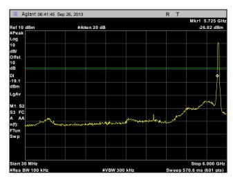
Plot 258. Conducted Spurious Emissions, Low Channel, 40 MHz, Port 2, 30 MHz - 6 GHz
