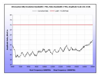
Plot 131. Radiated Spurious Emissions, High Channel, 20 MHz, 6 GHz – 18 GHz, Peak, 19 dBi
