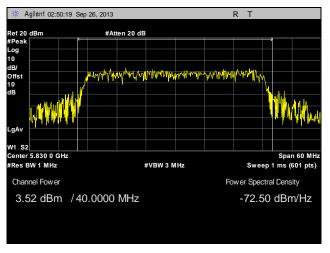
Plot 101. Peak Power Output, Point to Multi-Point, High Channel, 40 MHz, Port 2, 28 dBi
