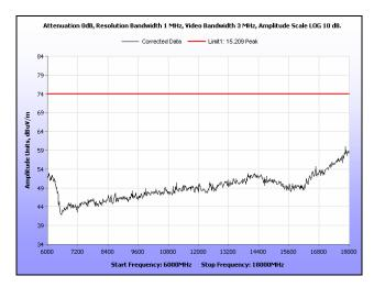
Plot 119. Radiated Spurious Emissions, High Channel, 20 MHz, 6 GHz - 18 GHz, Peak, 16 dBi
