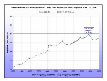
Plot 220. Radiated Spurious Emissions, Mid Channel, 40 MHz, 1 GHz - 6 GHz, Average, 28 dBi
