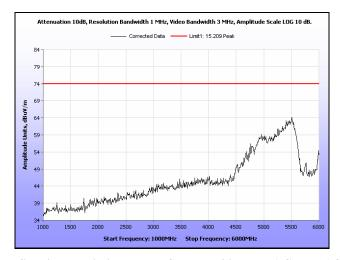
Plot 121. Radiated Spurious Emissions, Low Channel, 20 MHz, 1 GHz - 6 GHz, Peak, 19 dBi
