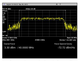
Plot 100. Peak Power Output, Point to Multi-Point, Mid Channel, 40 MHz, Port 2, 28 dBi
