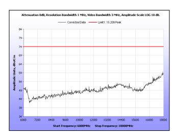
Plot 171. Radiated Spurious Emissions, Low Channel, 40 MHz, 6 GHz - 18 GHz, Peak, 16 dBi
