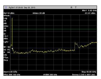
Plot 249. Conducted Spurious Emissions, Mid Channel, 20 MHz, Port 2, 5 GHz - 40 GHz
