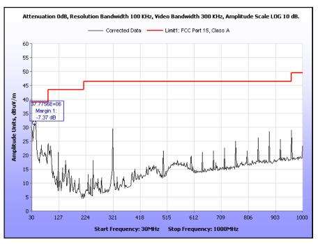
Plot 3. Radiated Emissions, 30 MHz - 1 GHz, FCC Limits
