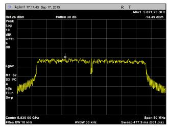
Plot 310. Peak Power Spectral Density, High Channel, Point to Multi-Point, 40 MHz, Port 1, 21 dBi
