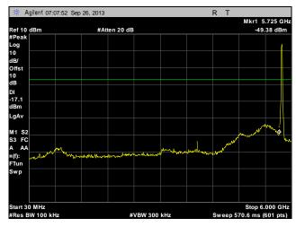
Plot 248. Conducted Spurious Emissions, Mid Channel, 20 MHz, Port 2, 30 MHz – 6 GHz
