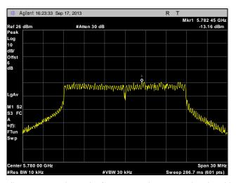
Plot 294. Peak Power Spectral Density, Mid Channel, Point to Multi-Point, 20 MHz, Port 2, 21 dBi
