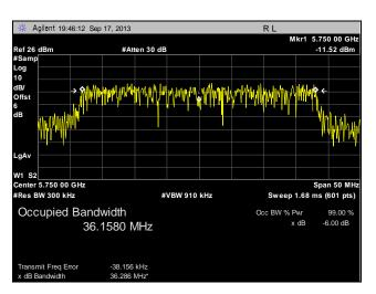
Plot 39. 99% Occupied Bandwidth, Low Channel, 40 MHz, Port 2
