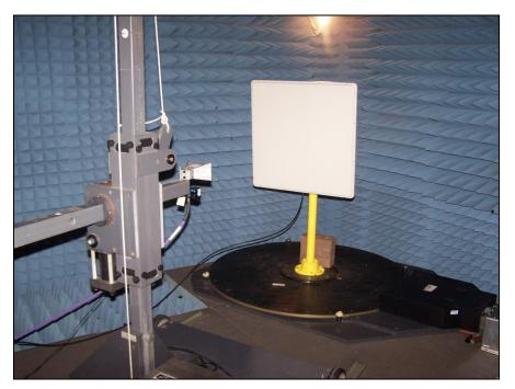
Photograph 7. Radiated Spurious Emissions, Test Setup, 18 GHz – 40 GHz
