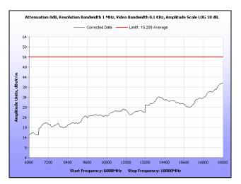
Plot 190. Radiated Spurious Emissions, High Channel, 40 MHz, 6 GHz - 18 GHz, Average, 19 dBi
