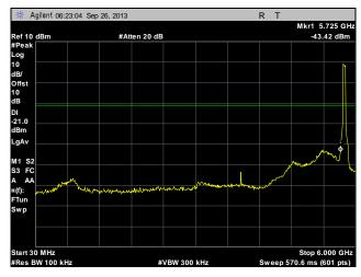
Plot 242. Conducted Spurious Emissions, Mid Channel, 20 MHz, Port 1, 30 MHz – 6 GHz
