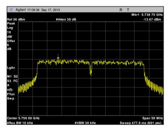
Plot 302. Peak Power Spectral Density, Low Channel, Point to Multi-Point, 40 MHz, Port 1, 16 dBi
