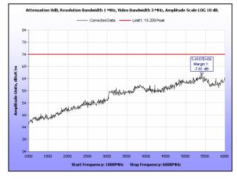
Plot 221. Radiated Spurious Emissions, Mid Channel, 40 MHz, 1 GHz - 6 GHz, Peak, 28 dBi
