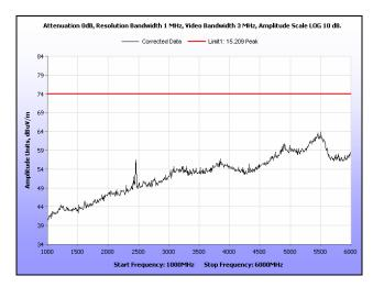
Plot 113. Radiated Spurious Emissions, Mid Channel, 20 MHz, 1 GHz - 6 GHz, Peak, 16 dBi
