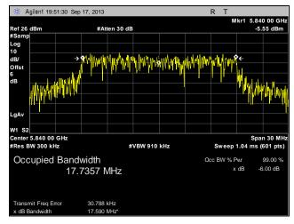
Plot 35. 99% Occupied Bandwidth, High Channel, 20 MHz, Port 2
