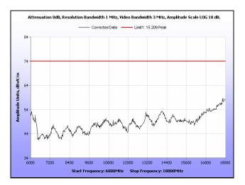
Plot 127. Radiated Spurious Emissions, Mid Channel, 20 MHz, 6 GHz - 18 GHz, Peak, 19 dBi
