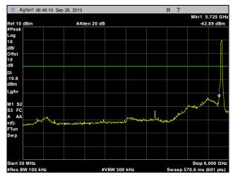
Plot 260. Conducted Spurious Emissions, Mid Channel, 40 MHz, Port 2, 30 MHz – 6 GHz
