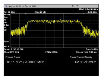
Plot 60. Peak Power Output, Point to Multi-Point, Low Channel, 20 MHz, Port 2, 19 dBi
