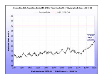
Plot 159. Radiated Spurious Emissions, Low Channel, 20 MHz, 6 GHz - 18 GHz, Peak, 28 dBi
