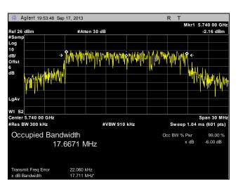
Plot 33. 99% Occupied Bandwidth, Low Channel, 20 MHz, Port 2
