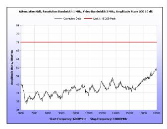
Plot 215. Radiated Spurious Emissions, High Channel, 40 MHz, 6 GHz – 18 GHz, Peak, 23 dBi
