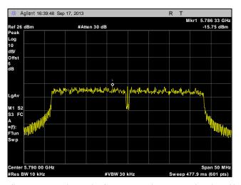
Plot 324. Peak Power Spectral Density, Mid Channel, Point to Multi-Point, 40 MHz, Port 2, 21 dBi
