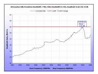
Plot 184. Radiated Spurious Emissions, Mid Channel, 40 MHz, 1 GHz - 6 GHz, Average, 19 dBi
