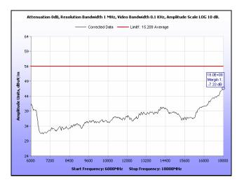
Plot 178. Radiated Spurious Emissions, High Channel, 40 MHz, 6 GHz - 18 GHz, Average, 16 dBi
