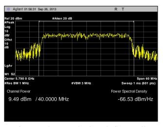
Plot 94. Peak Power Output, Point to Multi-Point, Mid Channel, 40 MHz, Port 2, 21 dBi
