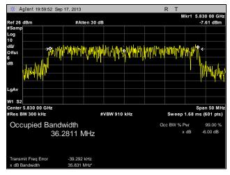
Plot 38. 99% Occupied Bandwidth, High Channel, 40 MHz, Port 1
