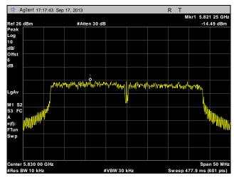
Plot 307. Peak Power Spectral Density, High Channel, Point to Multi-Point, 40 MHz, Port 1, 19 dBi
