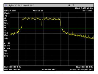
Plot 271. Conducted Band Edge, High Channel, 40 MHz, Port 2
