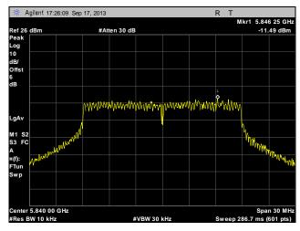
Plot 274. Peak Power Spectral Density, High Channel, Point to Multi-Point, 20 MHz, Port 1, 16 dBi
