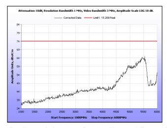
Plot 181. Radiated Spurious Emissions, Low Channel, 40 MHz, 1 GHz - 6 GHz, Peak, 19 dBi
