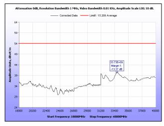
Plot 236. Radiated Spurious Emissions, Mid Channel, 40 MHz, 18 GHz – 40 GHz, Average
