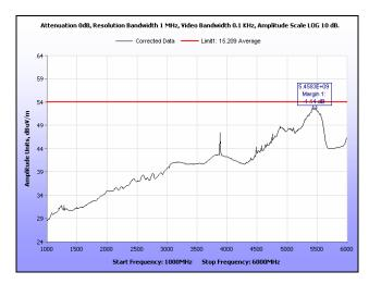
Plot 176. Radiated Spurious Emissions, High Channel, 40 MHz, 1 GHz - 6 GHz, Average, 16 dBi
