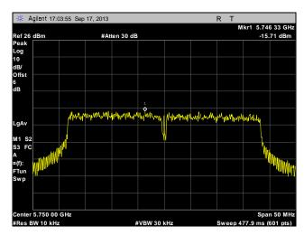
Plot 323. Peak Power Spectral Density, Low Channel, Point to Multi-Point, 40 MHz, Port 2, 21 dBi
