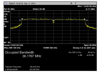
Plot 29. 6 dB Occupied Bandwidth, High Channel, 40 MHz, Port 2
