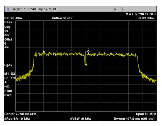
Plot 318. Peak Power Spectral Density, Mid Channel, Point to Multi-Point, 40 MHz, Port 2, 16 dBi
