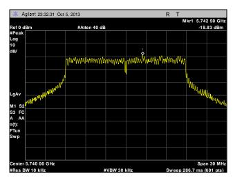
Plot 299. Peak Power Spectral Density, Low Channel, Point to Multi-Point, 20 MHz, Port 2, 28 dBi
