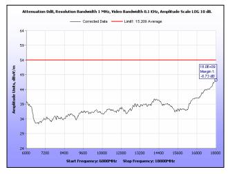
Plot 110. Radiated Spurious Emissions, Low Channel, 20 MHz, 6 GHz - 18 GHz, Average, 16 dBi
