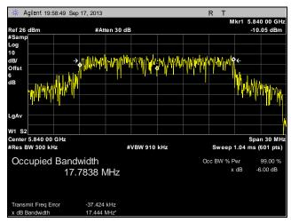
Plot 32. 99% Occupied Bandwidth, High Channel, 20 MHz, Port 1
