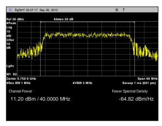
Plot 72. Peak Power Output, Point to Multi-Point, Low Channel, 40 MHz, Port 1, 16 dBi
