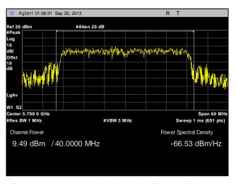
Plot 91. Peak Power Output, Point to Multi-Point, Mid Channel, 40 MHz, Port 2, Port 2, 19 dBi
