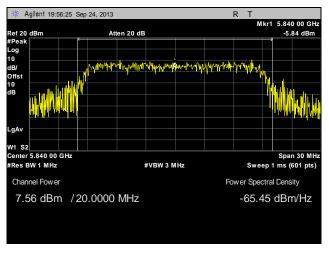
Plot 68. Peak Power Output, Point to Multi-Point, High Channel, 20 MHz, Port 2, 23 dBi
