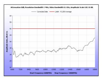
Plot 142. Radiated Spurious Emissions, High Channel, 20 MHz, 6 GHz - 18 GHz, Average, 21 dBi
