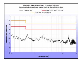
Plot 16. Conducted Emissions, 15.207(a), Neutral Line, Mid Channel, 40 MHz
