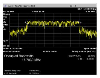
Plot 31. 99% Occupied Bandwidth, Mid Channel, 20 MHz, Port 1
