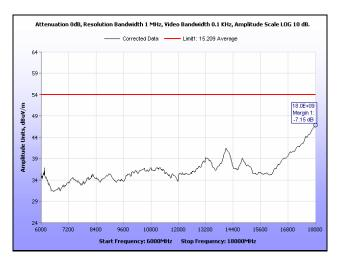
Plot 226. Radiated Spurious Emissions, High Channel, 40 MHz, 6 GHz - 18 GHz, Peak, 28 dBi
