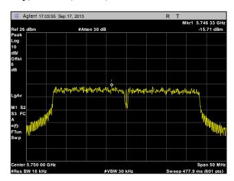
Plot 326. Peak Power Spectral Density, Low Channel, Point to Multi-Point, 40 MHz, Port 2, 23 dBi
