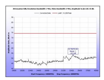
Plot 237. Radiated Spurious Emissions, Mid Channel, 40 MHz, 18 GHz – 40 GHz, Peak
