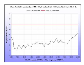
Plot 186. Radiated Spurious Emissions, Mid Channel, 40 MHz, 6 GHz – 18 GHz, Average, 19 dBi
