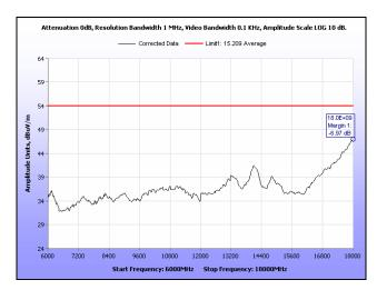
Plot 158. Radiated Spurious Emissions, Low Channel, 20 MHz, 6 GHz - 18 GHz, Average, 28 dBi
