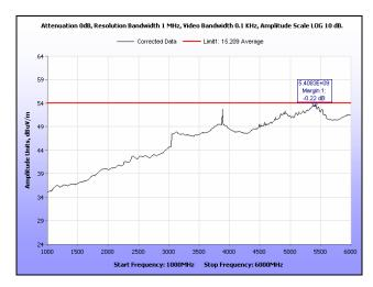
Plot 224. Radiated Spurious Emissions, High Channel, 40 MHz, 1 GHz – 6 GHz, Average, 28 dBi
