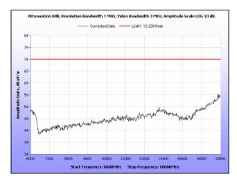
Plot 179. Radiated Spurious Emissions, High Channel, 40 MHz, 6 GHz – 18 GHz, Peak, 16 dBi
