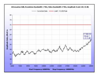
Plot 223. Radiated Spurious Emissions, Mid Channel, 40 MHz, 6 GHz - 18 GHz, Peak, 28 dBi
