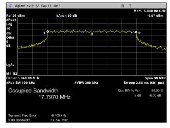
Plot 23. 6 dB Occupied Bandwidth, High Channel, 20 MHz, Port 2
