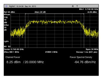
Plot 51. Peak Power Output, Point to Multi-Point, Low Channel, 20 MHz, Port 1, 23 dBi
