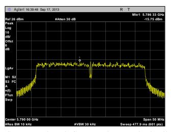
Plot 327. Peak Power Spectral Density, Mid Channel, Point to Multi-Point, 40 MHz, Port 2, 23 dBi
