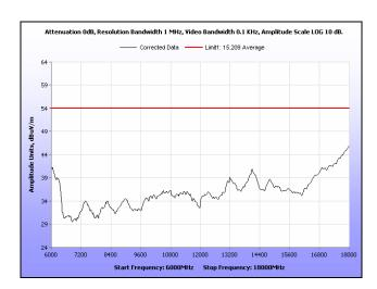
Plot 126. Radiated Spurious Emissions, Mid Channel, 20 MHz, 6 GHz – 18 GHz, Average, 19 dBi
