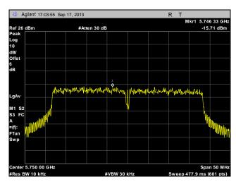
Plot 317. Peak Power Spectral Density, Low Channel, Point to Multi-Point, 40 MHz, Port 2, 16 dBi
