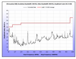
Plot 104. Radiated Spurious Emissions, High Channel, 20 MHz, 30 MHz - 1 GHz, Peak
