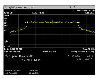
Plot 21. 6 dB Occupied Bandwidth, Low Channel, 20 MHz, Port 2
