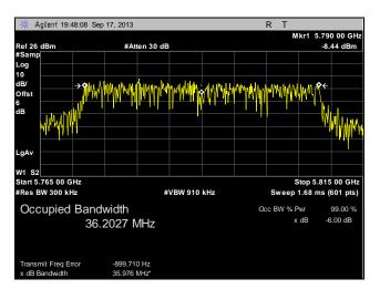
Plot 40. 99% Occupied Bandwidth, Mid Channel, 40 MHz, Port 2
