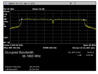
Plot 26. 6 dB Occupied Bandwidth, High Channel, 40 MHz, Port 1
