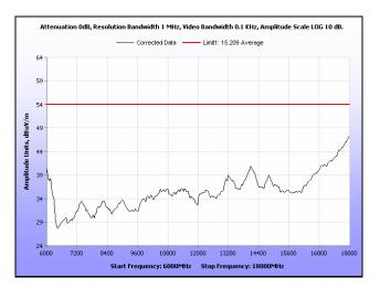
Plot 154. Radiated Spurious Emissions, High Channel, 20 MHz, 6 GHz - 18 GHz, Average, 23 dBi
