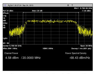
Plot 70. Peak Power Output, Point to Multi-Point, Mid Channel, 20 MHz, Port 2, 28 dBi
