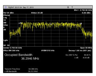
Plot 36. 99% Occupied Bandwidth, Low Channel, 40 MHz, Port 1
