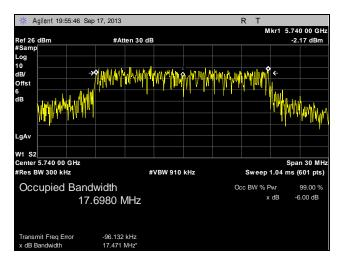
Plot 30. 99% Occupied Bandwidth, Low Channel, 20 MHz, Port 1
