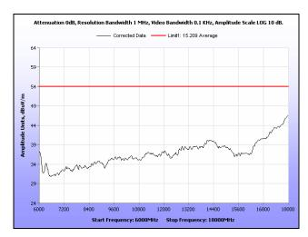
Plot 134. Radiated Spurious Emissions, Low Channel, 20 MHz, 6 GHz - 18 GHz, Average, 21 dBi
