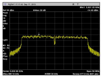
Plot 313. Peak Power Spectral Density, High Channel, Point to Multi-Point, 40 MHz, Port 1, 23 dBi
