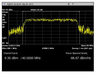
Plot 83. Peak Power Output, Point to Multi-Point, High Channel, 40 MHz, Port 1, 23 dBi
