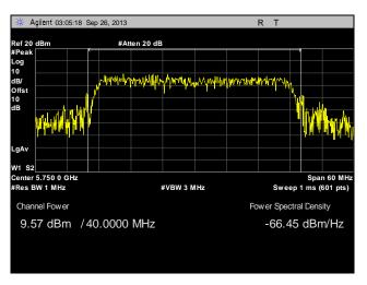
Plot 75. Peak Power Output, Point to Multi-Point, Low Channel, 40 MHz, Port 1, 19 dBi
