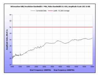
Plot 132. Radiated Spurious Emissions, Low Channel, 20 MHz, 1 GHz - 6 GHz, Average, 21 dBi
