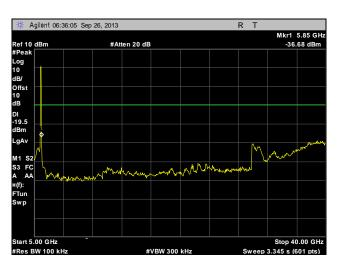
Plot 255. Conducted Spurious Emissions, Mid Channel, 40 MHz, Port 1, 5 GHz - 40 GHz
