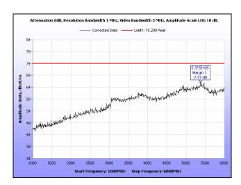
Plot 225. Radiated Spurious Emissions, High Channel, 40 MHz, 1 GHz - 6 GHz, Peak, 28 dBi
