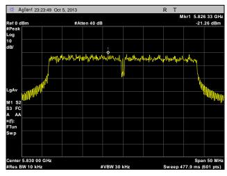
Plot 331. Peak Power Spectral Density, High Channel, Point to Multi-Point, 40 MHz, Port 2, 28 dBi
