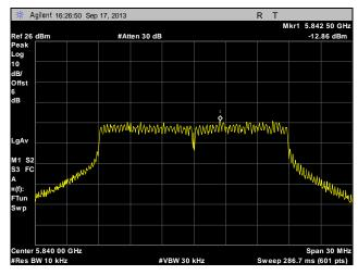
Plot 298. Peak Power Spectral Density, High Channel, Point to Multi-Point, 20 MHz, Port 2, 23 dBi
