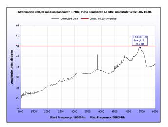
Plot 196. Radiated Spurious Emissions, Mid Channel, 40 MHz, 1 GHz - 6 GHz, Average, 21 dBi
