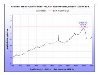
Plot 116. Radiated Spurious Emissions, High Channel, 20 MHz, 1 GHz - 6 GHz, Average, 16 dBi
