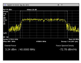
Plot 99. Peak Power Output, Point to Multi-Point, Low Channel, 40 MHz, Port 2, 28 dBi
