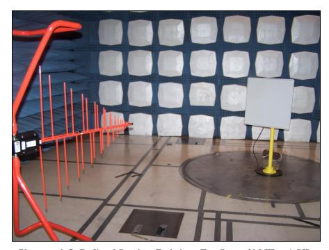
Photograph 5. Radiated Spurious Emissions, Test Setup, 30 MHz – 1 GHz
