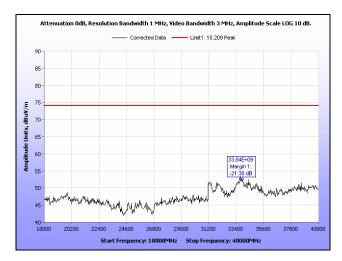
Plot 239. Radiated Spurious Emissions, High Channel, 40 MHz, 18 GHz - 40 GHz, Peak
