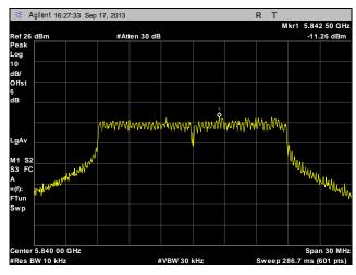
Plot 289. Peak Power Spectral Density, High Channel, Point to Multi-Point, 20 MHz, Port 2, 16 dBi
