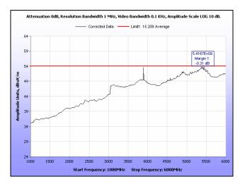
Plot 164. Radiated Spurious Emissions, High Channel, 20 MHz, 1 GHz - 6 GHz, Average, 28 dBi
