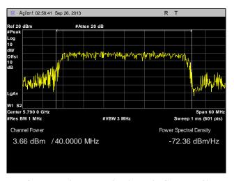
Plot 85. Peak Power Output, Point to Multi-Point, Mid Channel, 40 MHz, Port 1, 28 dBi
