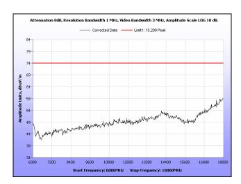
Plot 195. Radiated Spurious Emissions, Low Channel, 40 MHz, 6 GHz - 18 GHz, Peak, 21 dBi
