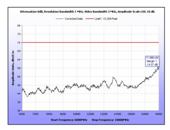
Plot 227. Radiated Spurious Emissions, High Channel, 40 MHz, 6 GHz – 18 GHz, Peak, 28 dBi
