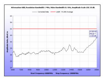
Plot 218. Radiated Spurious Emissions, Low Channel, 40 MHz, 6 GHz – 18 GHz, Peak, 28 dBi
