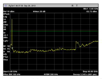
Plot 253. Conducted Spurious Emissions, Low Channel, 40 MHz, Port 1, 5 GHz - 40 GHz
