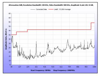
Plot 107. Radiated Spurious Emissions, High Channel, 40 MHz, 30 MHz - 1 GHz, Peak
