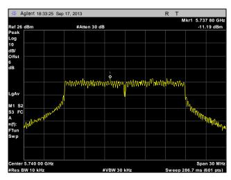
Plot 275. Peak Power Spectral Density, Low Channel, Point to Multi-Point, 20 MHz, Port 1, 19 dBi
