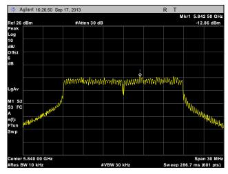
Plot 292. Peak Power Spectral Density, High Channel, Point to Multi-Point, 20 MHz, Port 2, 19 dBi
