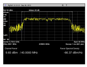
Plot 93. Peak Power Output, Point to Multi-Point, Low Channel, 40 MHz, Port 2, 21 dBi
