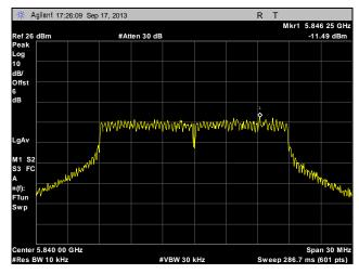
Plot 277. Peak Power Spectral Density, High Channel, Point to Multi-Point, 20 MHz, Port 1, 19 dBi
