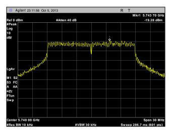
Plot 284. Peak Power Spectral Density, Low Channel, Point to Multi-Point, 20 MHz, Port 1, 28 dBi
