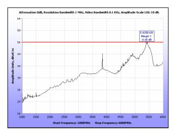
Plot 136. Radiated Spurious Emissions, Mid Channel, 20 MHz, 1 GHz - 6 GHz, Average, 21 dBi
