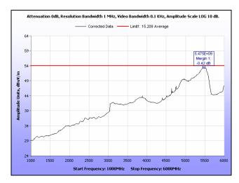
Plot 188. Radiated Spurious Emissions, High Channel, 40 MHz, 1 GHz - 6 GHz, Average, 19 dBi
