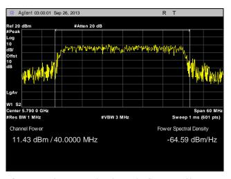
Plot 73. Peak Power Output, Point to Multi-Point, Mid Channel, 40 MHz, Port 1, Port 1, 16 dBi
