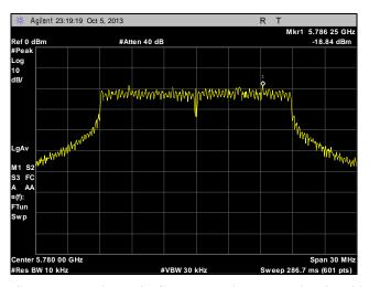
Plot 285. Peak Power Spectral Density, Mid Channel, Point to Multi-Point, 20 MHz, Port 1, 28 dBi
