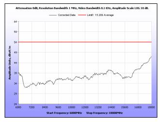
Plot 170. Radiated Spurious Emissions, Low Channel, 40 MHz, 6 GHz - 18 GHz, Average, 16 dBi
