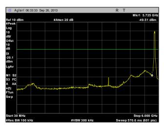
Plot 256. Conducted Spurious Emissions, High Channel, 40 MHz, Port 1, 30 MHz - 6 GHz
