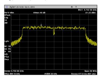
Plot 314. Peak Power Spectral Density, Low Channel, Point to Multi-Point, 40 MHz, Port 1, 28 dBi
