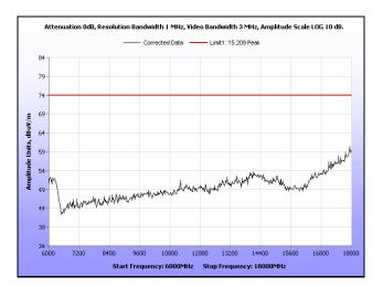
Plot 175. Radiated Spurious Emissions, Mid Channel, 40 MHz, 6 GHz - 18 GHz, Peak, 16 dBi
