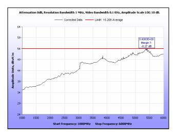
Plot 160. Radiated Spurious Emissions, Mid Channel, 20 MHz, 1 GHz - 6 GHz, Average, 28 dBi
