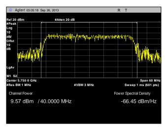
Plot 78. Peak Power Output, Point to Multi-Point, Low Channel, 40 MHz, Port 1, 21 dBi
