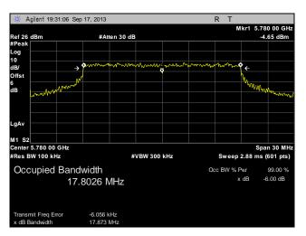
Plot 22. 6 dB Occupied Bandwidth, Mid Channel, 20 MHz, Port 2
