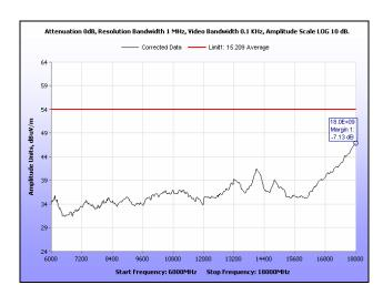
Plot 222. Radiated Spurious Emissions, Mid Channel, 40 MHz, 6 GHz - 18 GHz, Peak, 28 dBi
