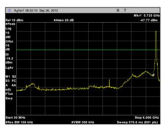
Plot 262. Conducted Spurious Emissions, High Channel, 40 MHz, Port 2, 30 MHz - 6 GHz
