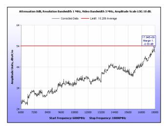
Plot 191. Radiated Spurious Emissions, High Channel, 40 MHz, 6 GHz - 18 GHz, Peak, 19 dBi
