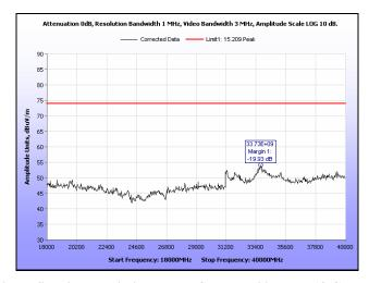
Plot 229. Radiated Spurious Emissions, Low Channel, 20 MHz, 18 GHz - 40 GHz, Peak
