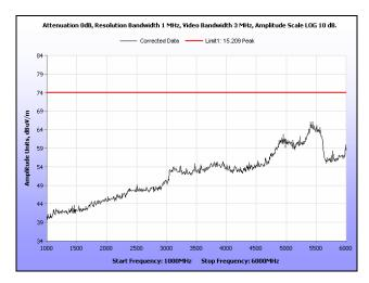
Plot 149. Radiated Spurious Emissions, Mid Channel, 20 MHz, 1 GHz - 6 GHz, Peak, 23 dBi
