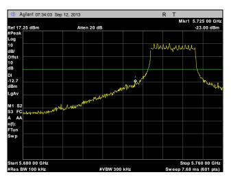
Plot 264. Conducted Band Edge, Low Channel, 20 MHz, Port 1
