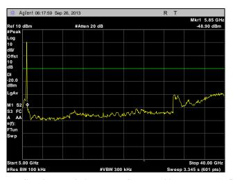
Plot 241. Conducted Spurious Emissions, Low Channel, 20 MHz, Port 1, 5 GHz - 40 GHz
