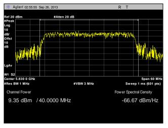
Plot 80. Peak Power Output, Point to Multi-Point, High Channel, 40 MHz, Port 1, 21 dBi
