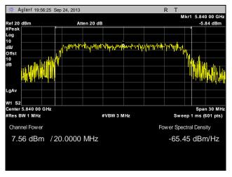
Plot 62. Peak Power Output, Point to Multi-Point, High Channel, 20 MHz, Port 2, Port 2, 19 dBi
