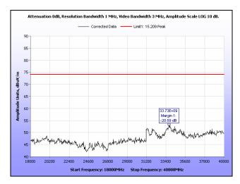
Plot 233. Radiated Spurious Emissions, High Channel, 20 MHz, 18 GHz - 40 GHz, Peak
