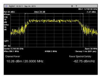
Plot 42. Peak Power Output, Point to Multi-Point, Low Channel, 20 MHz, Port 1, 16 dBi
