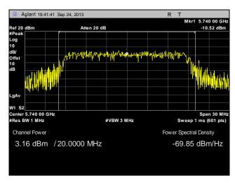
Plot 54. Peak Power Output, Point to Multi-Point, Low Channel, 20 MHz, Port 1, 28 dBi
