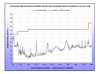
Plot 103. Radiated Spurious Emissions, Mid Channel, 20 MHz, 30 MHz - 1 GHz, Peak
