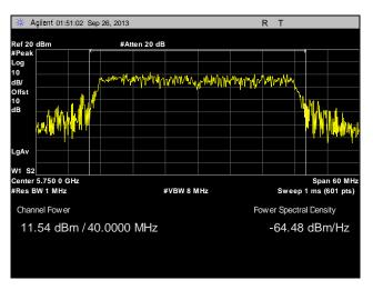
Plot 87. Peak Power Output, Point to Multi-Point, Low Channel, 40 MHz, Port 2, 16 dBi
