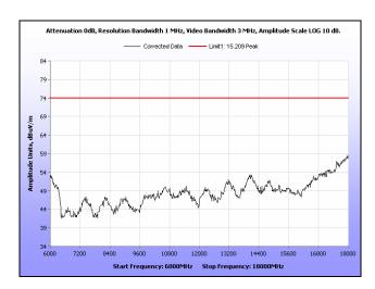
Plot 183. Radiated Spurious Emissions, Low Channel, 40 MHz, 6 GHz - 18 GHz, Peak, 19 dBi
