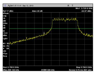
Plot 266. Conducted Band Edge, Low Channel, 20 MHz, Port 2
