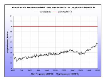
Plot 139. Radiated Spurious Emissions, Mid Channel, 20 MHz, 6 GHz - 18 GHz, Peak, 21 dBi
