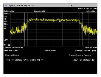
Plot 43. Peak Power Output, Point to Multi-Point, Mid Channel, 20 MHz, Port 1, Port 1, 16 dBi
