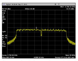
Plot 321. Peak Power Spectral Density, Mid Channel, Point to Multi-Point, 40 MHz, Port 2, 19 dBi
