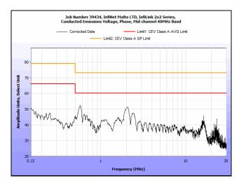
Plot 10. Conducted Emissions, 15.207(a), Phase Line, Mid Channel, 40 MHz
