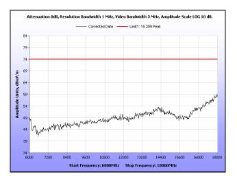
Plot 199. Radiated Spurious Emissions, Mid Channel, 40 MHz, 6 GHz - 18 GHz, Peak, 21 dBi
