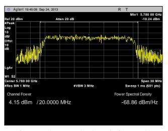
Plot 55. Peak Power Output, Point to Multi-Point, Mid Channel, 20 MHz, Port 1, 28 dBi
