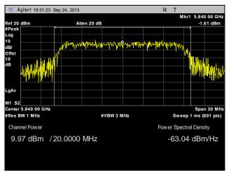
Plot 44. Peak Power Output, Point to Multi-Point, High Channel, 20 MHz, Port 1, Port 1, 16 dBi
