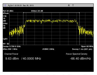
Plot 79. Peak Power Output, Point to Multi-Point, Mid Channel, 40 MHz, Port 1, 21 dBi
