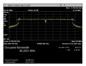
Plot 28. 6 dB Occupied Bandwidth, Mid Channel, 40 MHz, Port 2
