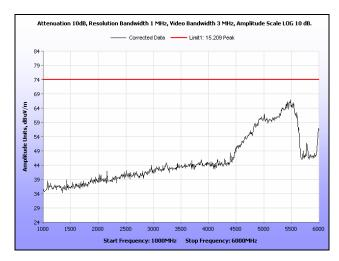
Plot 185. Radiated Spurious Emissions, Mid Channel, 40 MHz, 1 GHz - 6 GHz, Peak, 19 dBi
