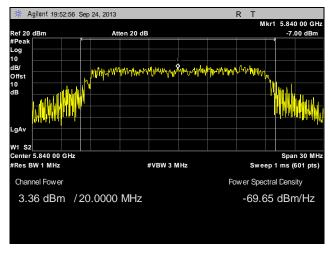
Plot 56. Peak Power Output, Point to Multi-Point, High Channel, 20 MHz, Port 1, 28 dBi
