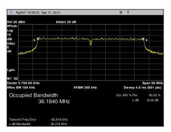
Plot 24. 6 dB Occupied Bandwidth, Low Channel, 40 MHz, Port 1
