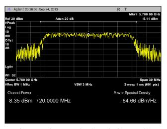
Plot 67. Peak Power Output, Point to Multi-Point, Mid Channel, 20 MHz, Port 2, 23 dBi
