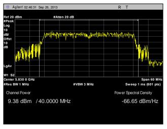
Plot 95. Peak Power Output, Point to Multi-Point, High Channel, 40 MHz, Port 2, 21 dBi
