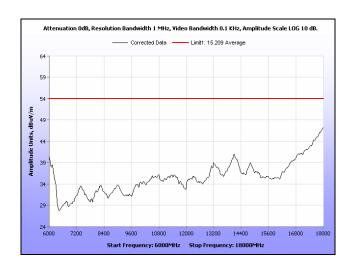
Plot 210. Radiated Spurious Emissions, Mid Channel, 40 MHz, 6 GHz – 18 GHz, Average, 23 dBi
