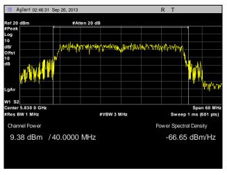
Plot 92. Peak Power Output, Point to Multi-Point, High Channel, 40 MHz, Port 2, Port 2, 19 dBi
