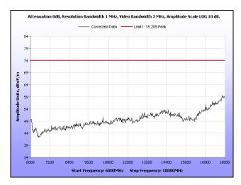
Plot 143. Radiated Spurious Emissions, High Channel, 20 MHz, 6 GHz – 18 GHz, Peak, 21 dBi
