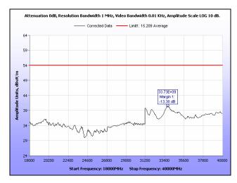
Plot 228. Radiated Spurious Emissions, Low Channel, 20 MHz, 18 GHz - 40 GHz, Average
