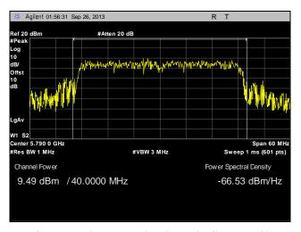
Plot 97. Peak Power Output, Point to Multi-Point, Mid Channel, 40 MHz, Port 2, 23 dBi
