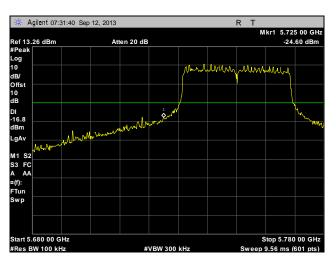
Plot 268. Conducted Band Edge, Low Channel, 40 MHz, Port 1
