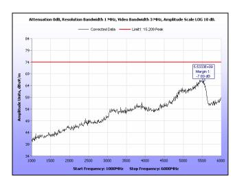
Plot 129. Radiated Spurious Emissions, High Channel, 20 MHz, 1 GHz - 6 GHz, Peak, 19 dBi
