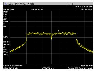
Plot 295. Peak Power Spectral Density, High Channel, Point to Multi-Point, 20 MHz, Port 2, 21 dBi
