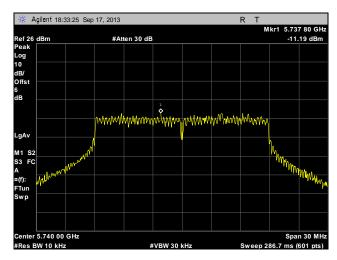
Plot 278. Peak Power Spectral Density, Low Channel, Point to Multi-Point, 20 MHz, Port 1, 21 dBi
