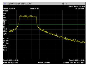
Plot 265. Conducted Band Edge, High Channel, 20 MHz, Port 1
