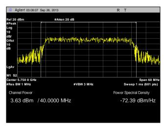
Plot 84. Peak Power Output, Point to Multi-Point, Low Channel, 40 MHz, Port 1, 28 dBi
