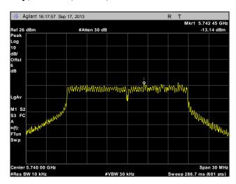
Plot 296. Peak Power Spectral Density, Low Channel, Point to Multi-Point, 20 MHz, Port 2, 23 dBi
