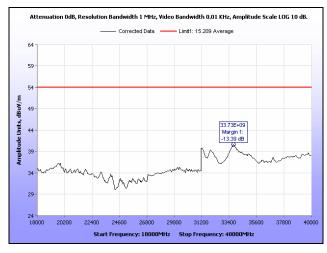
Plot 230. Radiated Spurious Emissions, Mid Channel, 20 MHz, 18 GHz - 40 GHz, Average
