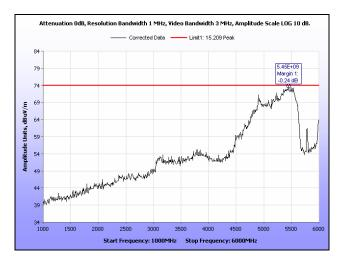
Plot 125. Radiated Spurious Emissions, Mid Channel, 20 MHz, 1 GHz - 6 GHz, Peak, 19 dBi
