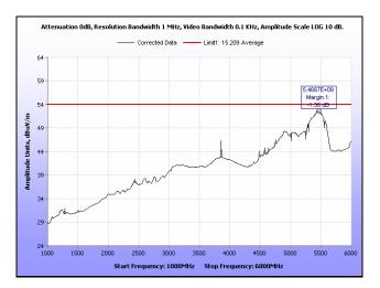
Plot 172. Radiated Spurious Emissions, Mid Channel, 40 MHz, 1 GHz - 6 GHz, Average, 16 dBi
