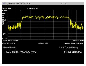
Plot 74. Peak Power Output, Point to Multi-Point, High Channel, 40 MHz, Port 1, Port 1, 16 dBi
