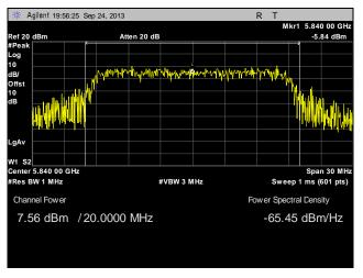
Plot 65. Peak Power Output, Point to Multi-Point, High Channel, 20 MHz, Port 2, 21 dBi
