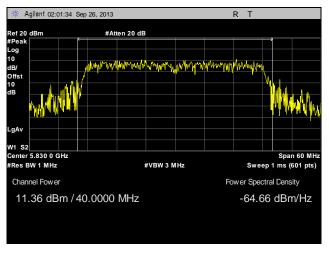
Plot 89. Peak Power Output, Point to Multi-Point, High Channel, 40 MHz, Port 2, Port 2, 16 dBi
