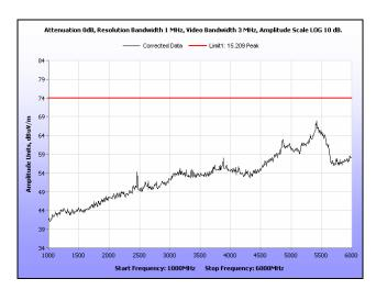
Plot 201. Radiated Spurious Emissions, High Channel, 40 MHz, 1 GHz - 6 GHz, Peak, 21 dBi
