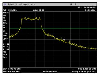
Plot 267. Conducted Band Edge, High Channel, 20 MHz, Port 2
