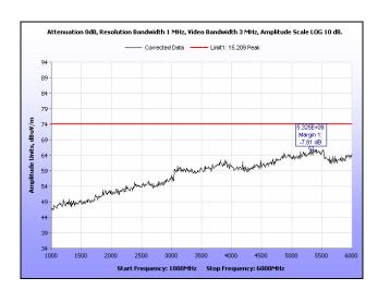
Plot 165. Radiated Spurious Emissions, High Channel, 20 MHz, 1 GHz - 6 GHz, Peak, 28 dBi
