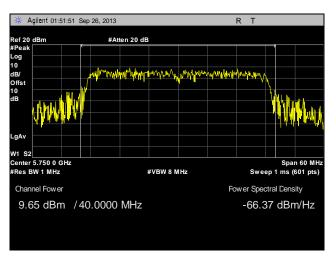
Plot 96. Peak Power Output, Point to Multi-Point, Low Channel, 40 MHz, Port 2, 23 dBi
