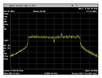
Plot 288. Peak Power Spectral Density, Mid Channel, Point to Multi-Point, 20 MHz, Port 2, 16 dBi
