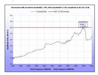
Plot 144. Radiated Spurious Emissions, Low Channel, 20 MHz, 1 GHz - 6 GHz, Average, 23 dBi
