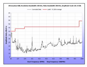
Plot 105. Radiated Spurious Emissions, Low Channel, 40 MHz, 30 MHz - 1 GHz, Peak
