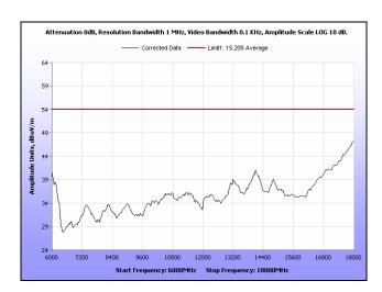
Plot 150. Radiated Spurious Emissions, Mid Channel, 20 MHz, 6 GHz – 18 GHz, Average, 23 dBi
