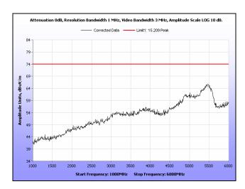
Plot 177. Radiated Spurious Emissions, High Channel, 40 MHz, 1 GHz - 6 GHz, Peak, 16 dBi
