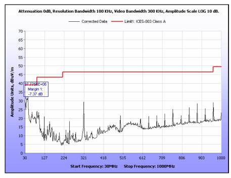
Plot 5. Radiated Emissions, 30 MHz - 1 GHz, ICES-003 Limits
