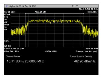
Plot 63. Peak Power Output, Point to Multi-Point, Low Channel, 20 MHz, Port 2, 21 dBi
