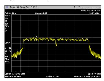
Plot 311. Peak Power Spectral Density, Low Channel, Point to Multi-Point, 40 MHz, Port 1, 23 dBi
