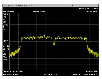
Plot 309. Peak Power Spectral Density, Mid Channel, Point to Multi-Point, 40 MHz, Port 1, 21 dBi
