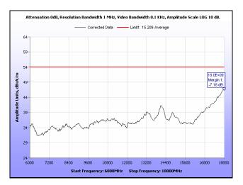
Plot 166. Radiated Spurious Emissions, High Channel, 20 MHz, 6 GHz - 18 GHz, Average, 28 dBi
