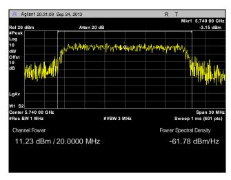
Plot 57. Peak Power Output, Point to Multi-Point, Low Channel, 20 MHz, Port 2, 16 dBi
