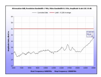
Plot 162. Radiated Spurious Emissions, Mid Channel, 20 MHz, 6 GHz – 18 GHz, Average, 28 dBi
