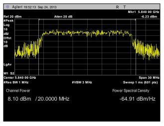
Plot 47. Peak Power Output, Point to Multi-Point, High Channel, 20 MHz, Port 1, Port 1, 19 dBi
