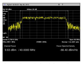
Plot 76. Peak Power Output, Point to Multi-Point, Mid Channel, 40 MHz, Port 1, Port 1, 19 dBi
