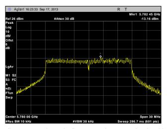
Plot 297. Peak Power Spectral Density, Mid Channel, Point to Multi-Point, 20 MHz, Port 2, 23 dBi
