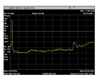
Plot 243. Conducted Spurious Emissions, Mid Channel, 20 MHz, Port 1, 5 GHz - 40 GHz
