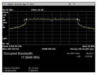
Plot 20. 6 dB Occupied Bandwidth, High Channel, 20 MHz, Port 1
