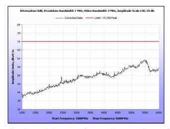
Plot 109. Radiated Spurious Emissions, Low Channel, 20 MHz, 1 GHz - 6 GHz, Peak, 16 dBi
