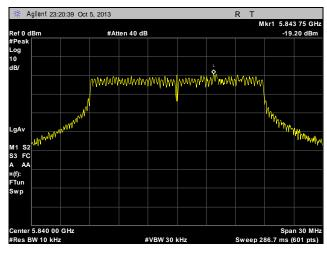
Plot 316. Peak Power Spectral Density, High Channel, Point to Multi-Point, 40 MHz, Port 1, 28 dBi
