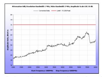
Plot 205. Radiated Spurious Emissions, Low Channel, 40 MHz, 1 GHz - 6 GHz, Peak, 23 dBi
