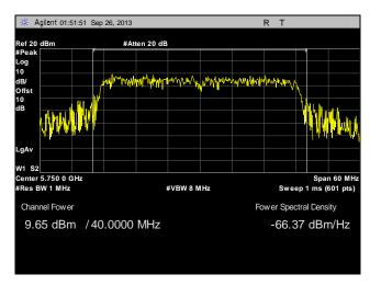
Plot 90. Peak Power Output, Point to Multi-Point, Low Channel, 40 MHz, Port 2, 19 dBi
