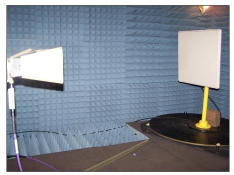
Photograph 6. Radiated Spurious Emissions, Test Setup, 1 GHz – 18 GHz
