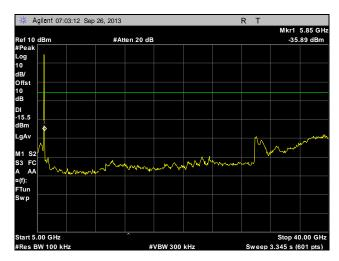
Plot 251. Conducted Spurious Emissions, High Channel, 20 MHz, Port 2, 5 GHz – 40 GHz
