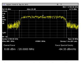
Plot 46. Peak Power Output, Point to Multi-Point, Mid Channel, 20 MHz, Port 1, Port 1, 19 dBi
