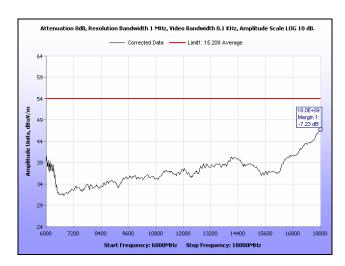
Plot 114. Radiated Spurious Emissions, Mid Channel, 20 MHz, 6 GHz – 18 GHz, Average, 16 dBi
