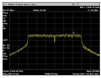
Plot 283. Peak Power Spectral Density, High Channel, Point to Multi-Point, 20 MHz, Port 1, 23 dBi
