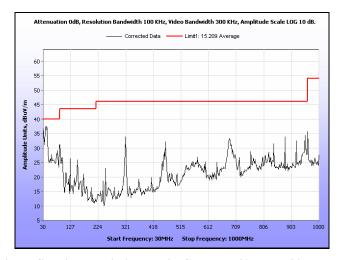
Plot 106. Radiated Spurious Emissions, Mid Channel, 40 MHz, 30 MHz - 1 GHz, Peak
