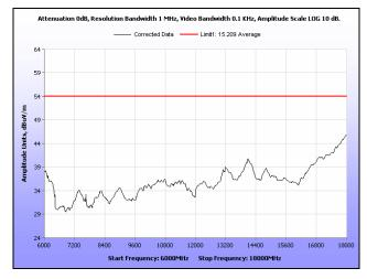
Plot 122. Radiated Spurious Emissions, Low Channel, 20 MHz, 6 GHz - 18 GHz, Average, 19 dBi
