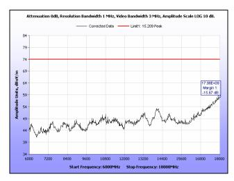
Plot 167. Radiated Spurious Emissions, High Channel, 20 MHz, 6 GHz – 18 GHz, Peak, 28 dBi
