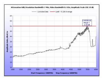
Plot 124. Radiated Spurious Emissions, Mid Channel, 20 MHz, 1 GHz - 6 GHz, Average, 19 dBi
