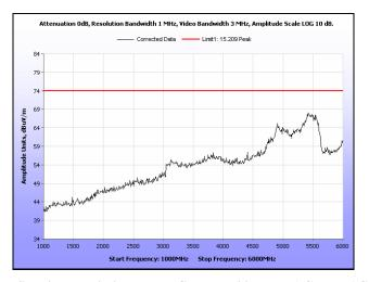
Plot 145. Radiated Spurious Emissions, Low Channel, 20 MHz, 1 GHz - 6 GHz, Peak, 23 dBi
