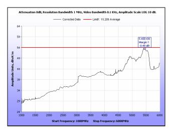
Plot 208. Radiated Spurious Emissions, Mid Channel, 40 MHz, 1 GHz - 6 GHz, Average, 23 dBi
