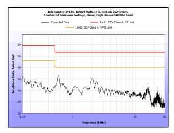
Plot 11. Conducted Emissions, 15.207(a), Phase Line, High Channel, 40 MHz
