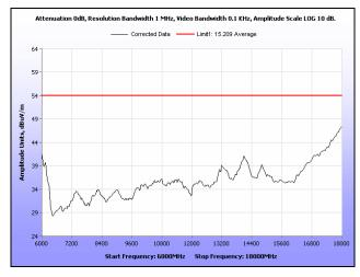
Plot 146. Radiated Spurious Emissions, Low Channel, 20 MHz, 6 GHz - 18 GHz, Average, 23 dBi
