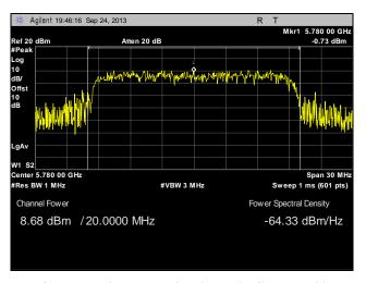
Plot 52. Peak Power Output, Point to Multi-Point, Mid Channel, 20 MHz, Port 1, 23 dBi
