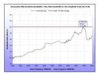
Plot 152. Radiated Spurious Emissions, High Channel, 20 MHz, 1 GHz - 6 GHz, Average, 23 dBi
