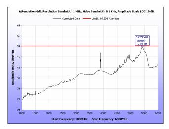
Plot 200. Radiated Spurious Emissions, High Channel, 40 MHz, 1 GHz - 6 GHz, Average, 21 dBi
