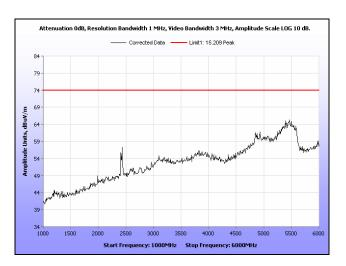
Plot 117. Radiated Spurious Emissions, High Channel, 20 MHz, 1 GHz - 6 GHz, Peak, 16 dBi
