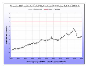
Plot 197. Radiated Spurious Emissions, Mid Channel, 40 MHz, 1 GHz - 6 GHz, Peak, 21 dBi
