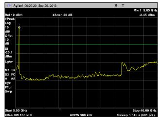
Plot 245. Conducted Spurious Emissions, High Channel, 20 MHz, Port 1, 5 GHz – 40 GHz
