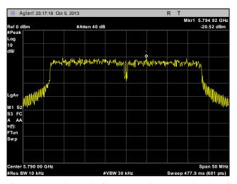
Plot 315. Peak Power Spectral Density, Mid Channel, Point to Multi-Point, 40 MHz, Port 1, 28 dBi
