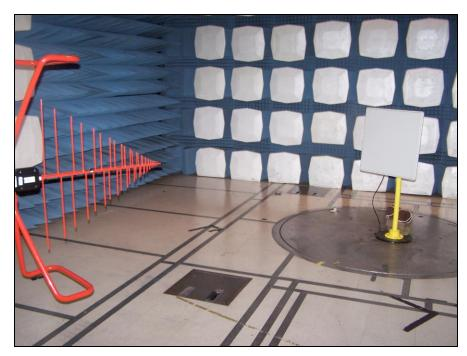
Photograph 3. Radiated Emissions, Test Setup, 30 MHz – 1 GHz
