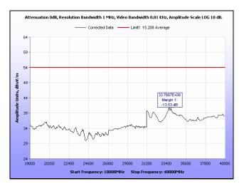
Plot 238. Radiated Spurious Emissions, High Channel, 40 MHz, 18 GHz - 40 GHz, Average
