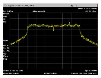
Plot 300. Peak Power Spectral Density, Mid Channel, Point to Multi-Point, 20 MHz, Port 2, 28 dBi
