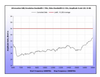
Plot 174. Radiated Spurious Emissions, Mid Channel, 40 MHz, 6 GHz - 18 GHz, Average, 16 dBi
