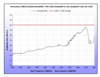
Plot 120. Radiated Spurious Emissions, Low Channel, 20 MHz, 1 GHz - 6 GHz, Average, 19 dBi
