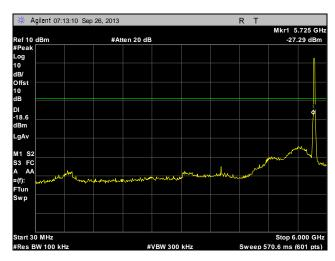
Plot 246. Conducted Spurious Emissions, Low Channel, 20 MHz, Port 2, 30 MHz - 6 GHz
