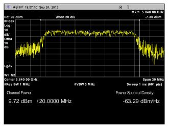
Plot 59. Peak Power Output, Point to Multi-Point, High Channel, 20 MHz, Port 2, Port 2, 16 dBi
