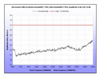
Plot 115. Radiated Spurious Emissions, Mid Channel, 20 MHz, 6 GHz - 18 GHz, Peak, 16 dBi
