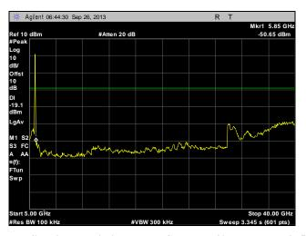
Plot 259. Conducted Spurious Emissions, Low Channel, 40 MHz, Port 2, 5 GHz – 40 GHz
