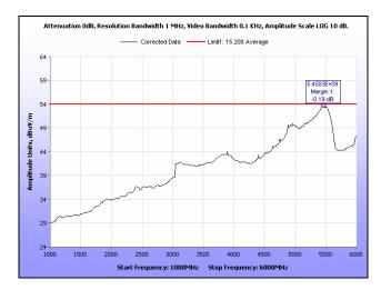
Plot 128. Radiated Spurious Emissions, High Channel, 20 MHz, 1 GHz – 6 GHz, Average, 19 dBi
