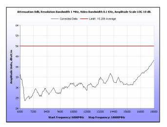
Plot 214. Radiated Spurious Emissions, High Channel, 40 MHz, 6 GHz - 18 GHz, Average, 23 dBi
