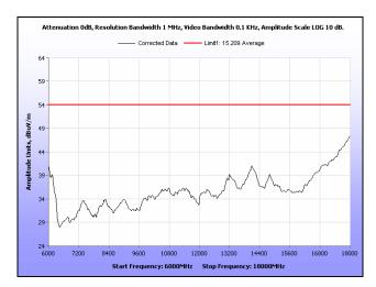
Plot 206. Radiated Spurious Emissions, Low Channel, 40 MHz, 6 GHz - 18 GHz, Average, 23 dBi
