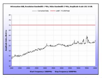
Plot 133. Radiated Spurious Emissions, Low Channel, 20 MHz, 1 GHz - 6 GHz, Peak, 21 dBi
