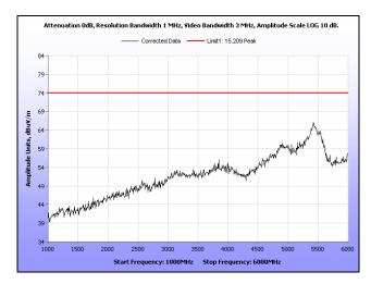
Plot 137. Radiated Spurious Emissions, Mid Channel, 20 MHz, 1 GHz - 6 GHz, Peak, 21 dBi
