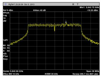
Plot 286. Peak Power Spectral Density, High Channel, Point to Multi-Point, 20 MHz, Port 1, 28 dBi
