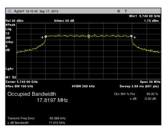
Plot 18. 6 dB Occupied Bandwidth, Low Channel, 20 MHz, Port 1
