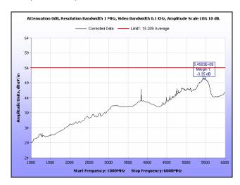
Plot 168. Radiated Spurious Emissions, Low Channel, 40 MHz, 1 GHz - 6 GHz, Average, 16 dBi
