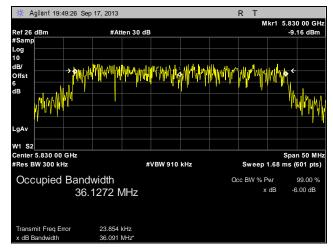
Plot 41. 99% Occupied Bandwidth, High Channel, 40 MHz, Port 2
