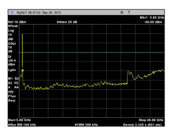
Plot 261. Conducted Spurious Emissions, Mid Channel, 40 MHz, Port 2, 5 GHz - 40 GHz
