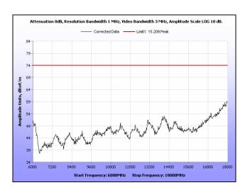
Plot 207. Radiated Spurious Emissions, Low Channel, 40 MHz, 6 GHz - 18 GHz, Peak, 23 dBi
