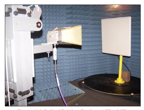
Photograph 4. Radiated Emissions, Test Setup, 1 GHz - 2 GHz
