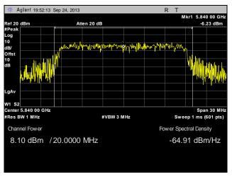
Plot 50. Peak Power Output, Point to Multi-Point, High Channel, 20 MHz, Port 1, 21 dBi
