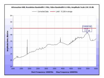
Plot 112. Radiated Spurious Emissions, Mid Channel, 20 MHz, 1 GHz - 6 GHz, Average, 16 dBi
