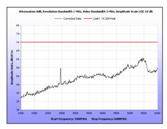
Plot 173. Radiated Spurious Emissions, Mid Channel, 40 MHz, 1 GHz - 6 GHz, Peak, 16 dBi
