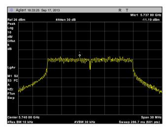
Plot 281. Peak Power Spectral Density, Low Channel, Point to Multi-Point, 20 MHz, Port 1, 23 dBi
