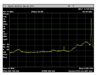
Plot 244. Conducted Spurious Emissions, High Channel, 20 MHz, Port 1, 30 MHz - 6 GHz
