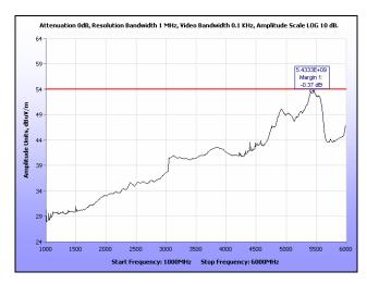
Plot 212. Radiated Spurious Emissions, High Channel, 40 MHz, 1 GHz - 6 GHz, Average, 23 dBi
