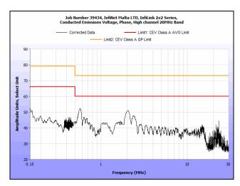
Plot 8. Conducted Emissions, 15.207(a), Phase Line, High Channel, 20 MHz
