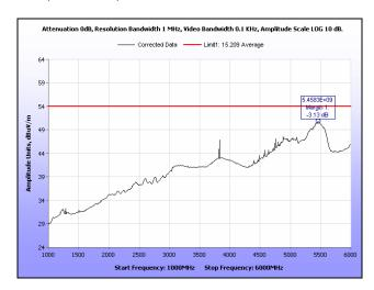
Plot 108. Radiated Spurious Emissions, Low Channel, 20 MHz, 1 GHz - 6 GHz, Average, 16 dBi
