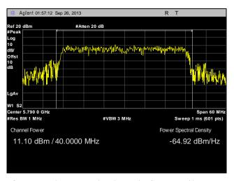
Plot 88. Peak Power Output, Point to Multi-Point, Mid Channel, 40 MHz, Port 2, Port 2, 16 dBi
