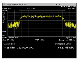
Plot 49. Peak Power Output, Point to Multi-Point, Mid Channel, 20 MHz, Port 1, 21 dBi
