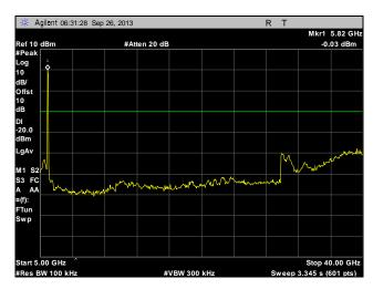
Plot 257. Conducted Spurious Emissions, High Channel, 40 MHz, Port 1, 5 GHz - 40 GHz
