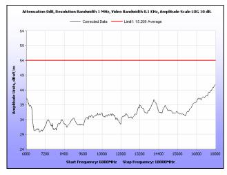
Plot 182. Radiated Spurious Emissions, Low Channel, 40 MHz, 6 GHz - 18 GHz, Average, 19 dBi
