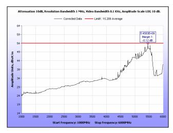
Plot 180. Radiated Spurious Emissions, Low Channel, 40 MHz, 1 GHz - 6 GHz, Average, 19 dBi
