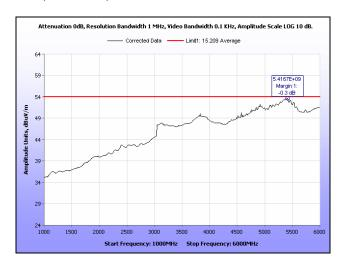
Plot 156. Radiated Spurious Emissions, Low Channel, 20 MHz, 1 GHz - 6 GHz, Average, 28 dBi
