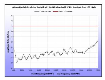
Plot 155. Radiated Spurious Emissions, High Channel, 20 MHz, 6 GHz – 18 GHz, Peak, 23 dBi
