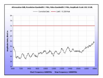
Plot 187. Radiated Spurious Emissions, Mid Channel, 40 MHz, 6 GHz - 18 GHz, Peak, 19 dBi
