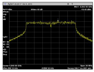
Plot 301. Peak Power Spectral Density, High Channel, Point to Multi-Point, 20 MHz, Port 2, 28 dBi
