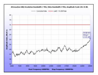
Plot 163. Radiated Spurious Emissions, Mid Channel, 20 MHz, 6 GHz - 18 GHz, Peak, 28 dBi
