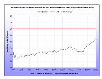
Plot 194. Radiated Spurious Emissions, Low Channel, 40 MHz, 6 GHz - 18 GHz, Average, 21 dBi
