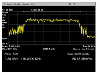
Plot 98. Peak Power Output, Point to Multi-Point, High Channel, 40 MHz, Port 2, 23 dBi
