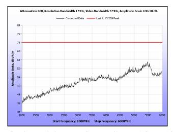
Plot 169. Radiated Spurious Emissions, Low Channel, 40 MHz, 1 GHz - 6 GHz, Peak, 16 dBi
