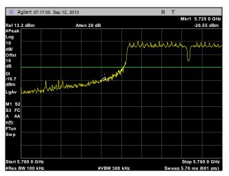
Plot 270. Conducted Band Edge, Low Channel, 40 MHz, Port 2
