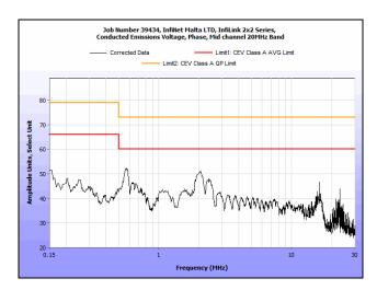
Plot 6. Conducted Emissions, 15.207(a), Phase Line, Low Channel, 20 MHz
