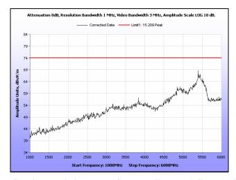
Plot 193. Radiated Spurious Emissions, Low Channel, 40 MHz, 1 GHz - 6 GHz, Peak, 21 dBi
