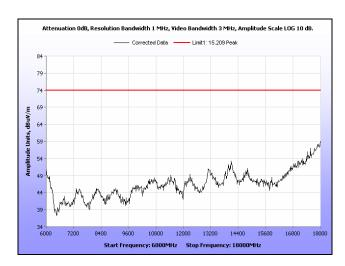
Plot 147. Radiated Spurious Emissions, Low Channel, 20 MHz, 6 GHz - 18 GHz, Peak, 23 dBi
