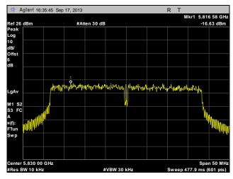
Plot 322. Peak Power Spectral Density, High Channel, Point to Multi-Point, 40 MHz, Port 2, 19 dBi
