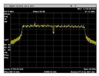
Plot 329. Peak Power Spectral Density, Low Channel, Point to Multi-Point, 40 MHz, Port 2, 28 dBi
