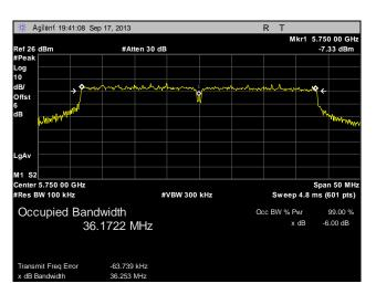
Plot 27. 6 dB Occupied Bandwidth, Low Channel, 40 MHz, Port 2
