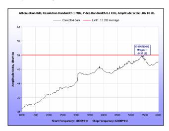
Plot 216. Radiated Spurious Emissions, Low Channel, 40 MHz, 1 GHz - 6 GHz, Average, 28 dBi
