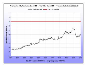
Plot 209. Radiated Spurious Emissions, Mid Channel, 40 MHz, 1 GHz - 6 GHz, Peak, 23 dBi
