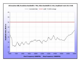
Plot 130. Radiated Spurious Emissions, High Channel, 20 MHz, 6 GHz - 18 GHz, Average, 19 dBi
