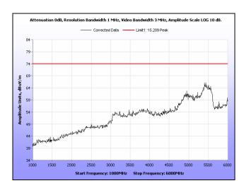
Plot 153. Radiated Spurious Emissions, High Channel, 20 MHz, 1 GHz - 6 GHz, Peak, 23 dBi
