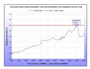
Plot 204. Radiated Spurious Emissions, Low Channel, 40 MHz, 1 GHz - 6 GHz, Average, 23 dBi
