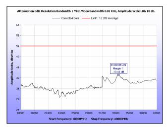
Plot 234. Radiated Spurious Emissions, Low Channel, 40 MHz, 18 GHz - 40 GHz, Average
