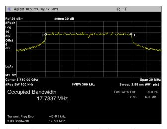
Plot 19. 6 dB Occupied Bandwidth, Mid Channel, 20 MHz, Port 1
