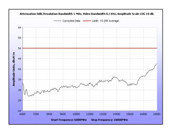
Plot 198. Radiated Spurious Emissions, Mid Channel, 40 MHz, 6 GHz - 18 GHz, Average, 21 dBi
