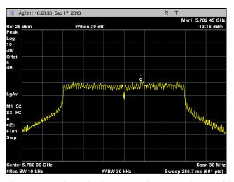
Plot 291. Peak Power Spectral Density, Mid Channel, Point to Multi-Point, 20 MHz, Port 2, 19 dBi
