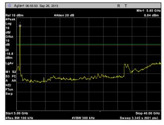
Plot 263. Conducted Spurious Emissions, High Channel, 40 MHz, Port 2, 5 GHz – 40 GHz
