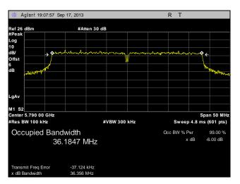
Plot 25. 6 dB Occupied Bandwidth, Mid Channel, 40 MHz, Port 1
