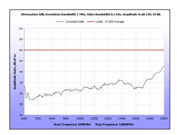
Plot 138. Radiated Spurious Emissions, Mid Channel, 20 MHz, 6 GHz – 18 GHz, Average, 21 dBi
