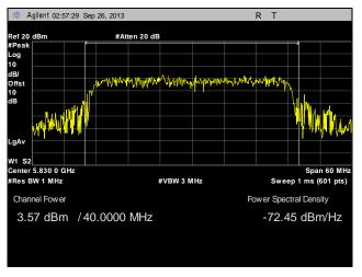
Plot 86. Peak Power Output, Point to Multi-Point, High Channel, 40 MHz, Port 1, 28 dBi
