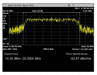
Plot 58. Peak Power Output, Point to Multi-Point, Mid Channel, 20 MHz, Port 2, Port 2, 16 dBi
