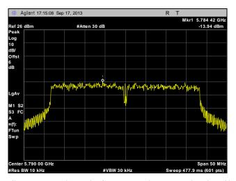
Plot 303. Peak Power Spectral Density, Mid Channel, Point to Multi-Point, 40 MHz, Port 1, 16 dBi
