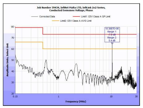
Plot 1. Conducted Emission, Phase Line Plot
