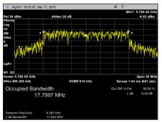
Plot 34. 99% Occupied Bandwidth, Mid Channel, 20 MHz, Port 2
