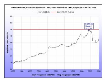
Plot 148. Radiated Spurious Emissions, Mid Channel, 20 MHz, 1 GHz - 6 GHz, Average, 23 dBi
