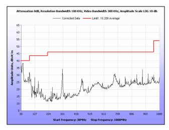
Plot 102. Radiated Spurious Emissions, Low Channel, 20 MHz, 30 MHz - 1 GHz, Peak
