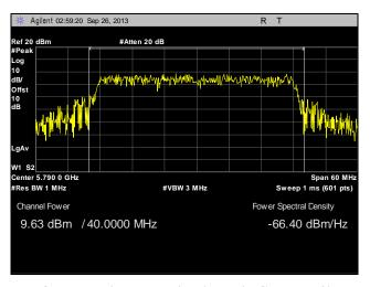
Plot 82. Peak Power Output, Point to Multi-Point, Mid Channel, 40 MHz, Port 1, 23 dBi
