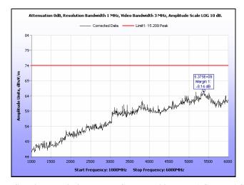
Plot 157. Radiated Spurious Emissions, Low Channel, 20 MHz, 1 GHz - 6 GHz, Peak, 28 dBi
