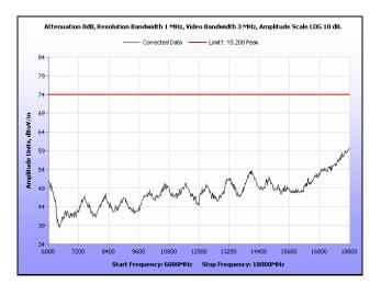
Plot 151. Radiated Spurious Emissions, Mid Channel, 20 MHz, 6 GHz - 18 GHz, Peak, 23 dBi
