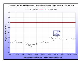
Plot 232. Radiated Spurious Emissions, High Channel, 20 MHz, 18 GHz - 40 GHz, Average
