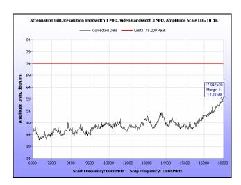
Plot 219. Radiated Spurious Emissions, Low Channel, 40 MHz, 6 GHz - 18 GHz, Peak, 28 dBi
