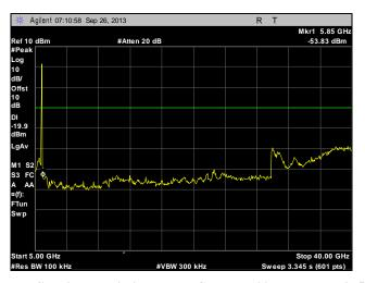
Plot 247. Conducted Spurious Emissions, Low Channel, 20 MHz, Port 2, 5 GHz - 40 GHz
