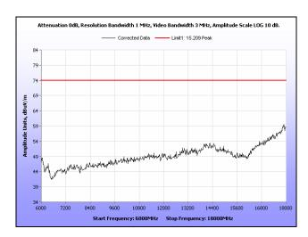
Plot 135. Radiated Spurious Emissions, Low Channel, 20 MHz, 6 GHz - 18 GHz, Peak, 21 dBi
