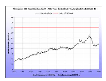
Plot 141. Radiated Spurious Emissions, High Channel, 20 MHz, 1 GHz - 6 GHz, Peak, 21 dBi
