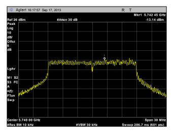
Plot 287. Peak Power Spectral Density, Low Channel, Point to Multi-Point, 20 MHz, Port 2, 16 dBi
