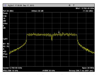
Plot 273. Peak Power Spectral Density, Mid Channel, Point to Multi-Point, 20 MHz, Port 1, 16 dBi
