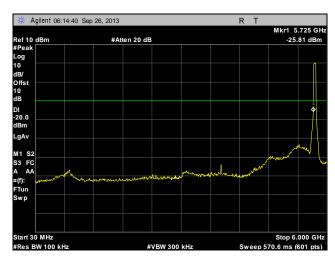
Plot 240. Conducted Spurious Emissions, Low Channel, 20 MHz, Port 1, 30 MHz - 6 GHz
