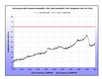
Plot 189. Radiated Spurious Emissions, High Channel, 40 MHz, 1 GHz - 6 GHz, Peak, 19 dBi
