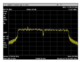
Plot 308. Peak Power Spectral Density, Low Channel, Point to Multi-Point, 40 MHz, Port 1, 21 dBi
