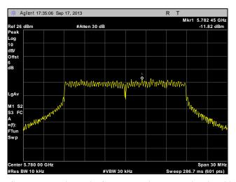
Plot 279. Peak Power Spectral Density, Mid Channel, Point to Multi-Point, 20 MHz, Port 1, 21 dBi
