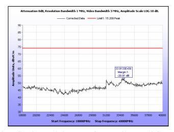
Plot 235. Radiated Spurious Emissions, Low Channel, 40 MHz, 18 GHz – 40 GHz, Peak
