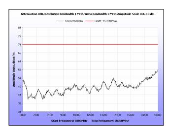
Plot 123. Radiated Spurious Emissions, Low Channel, 20 MHz, 6 GHz - 18 GHz, Peak, 19 dBi
