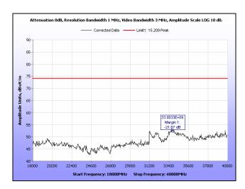
Plot 231. Radiated Spurious Emissions, Mid Channel, 20 MHz, 18 GHz – 40 GHz, Peak
