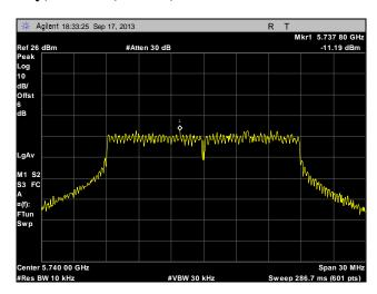
Plot 272. Peak Power Spectral Density, Low Channel, Point to Multi-Point, 20 MHz, Port 1, 16 dBi
